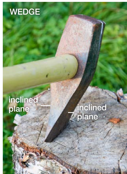
A wedge can split a piece of wood.
