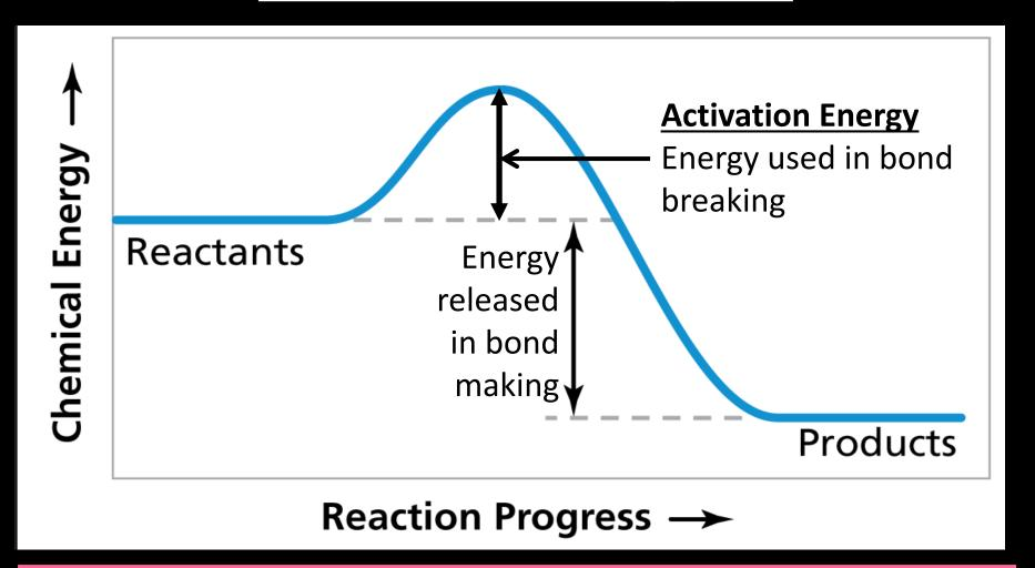
Exothermic - More energy is released when the products where formed than energy was used to break bonds in the reactants. Therefore, a net release of energy.
