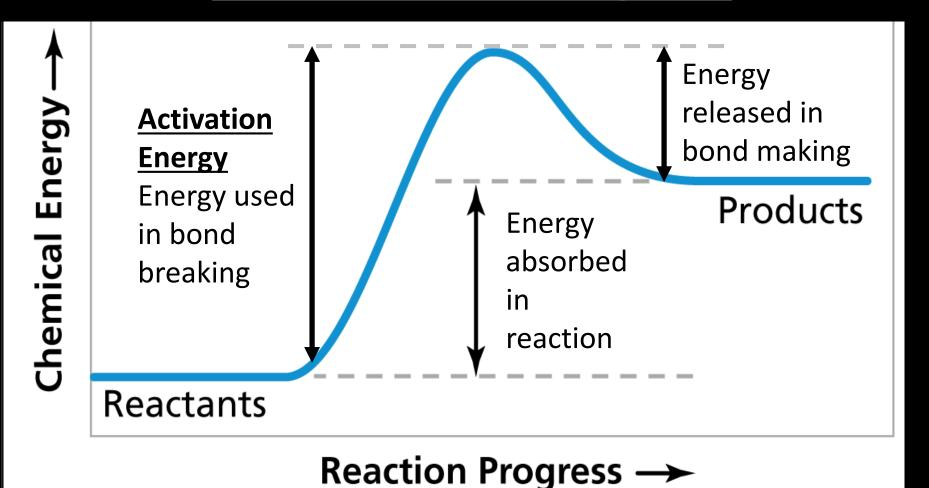
Endothermic - more energy is taken in to break the bonds in the reactants than released by the bonds being formed in the products. Therefore, energy is absorbed.
